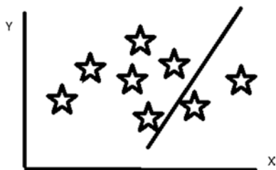
Fig. 8. Overgeneralization. This type of bias cannot capture the underlying trend of the data by underestimating the data. A linear function in the figure is used to perform the model; however, the model is unable to fit the training data well enough to learn with a good performance
