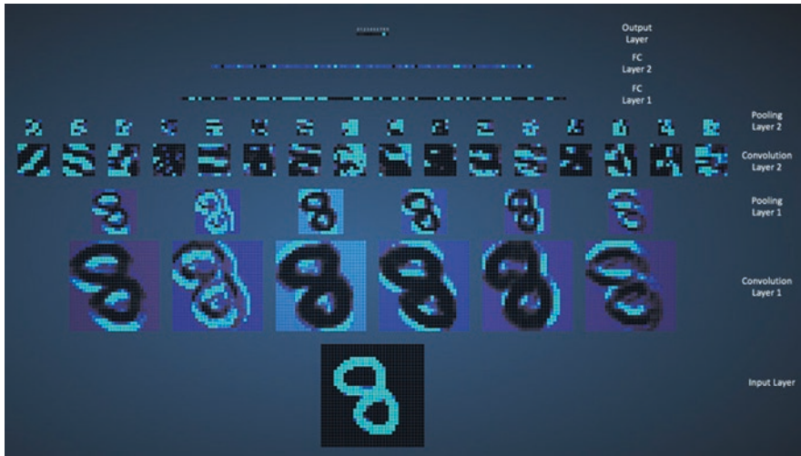
Fig. 10 A layer-by-layer breakdown of a convolutional neural network trained to recognize handwritten digits (Harley, 2015). As we go deeper into the network, the initial image is processed into simpler chunks before the number “8” is outputted
